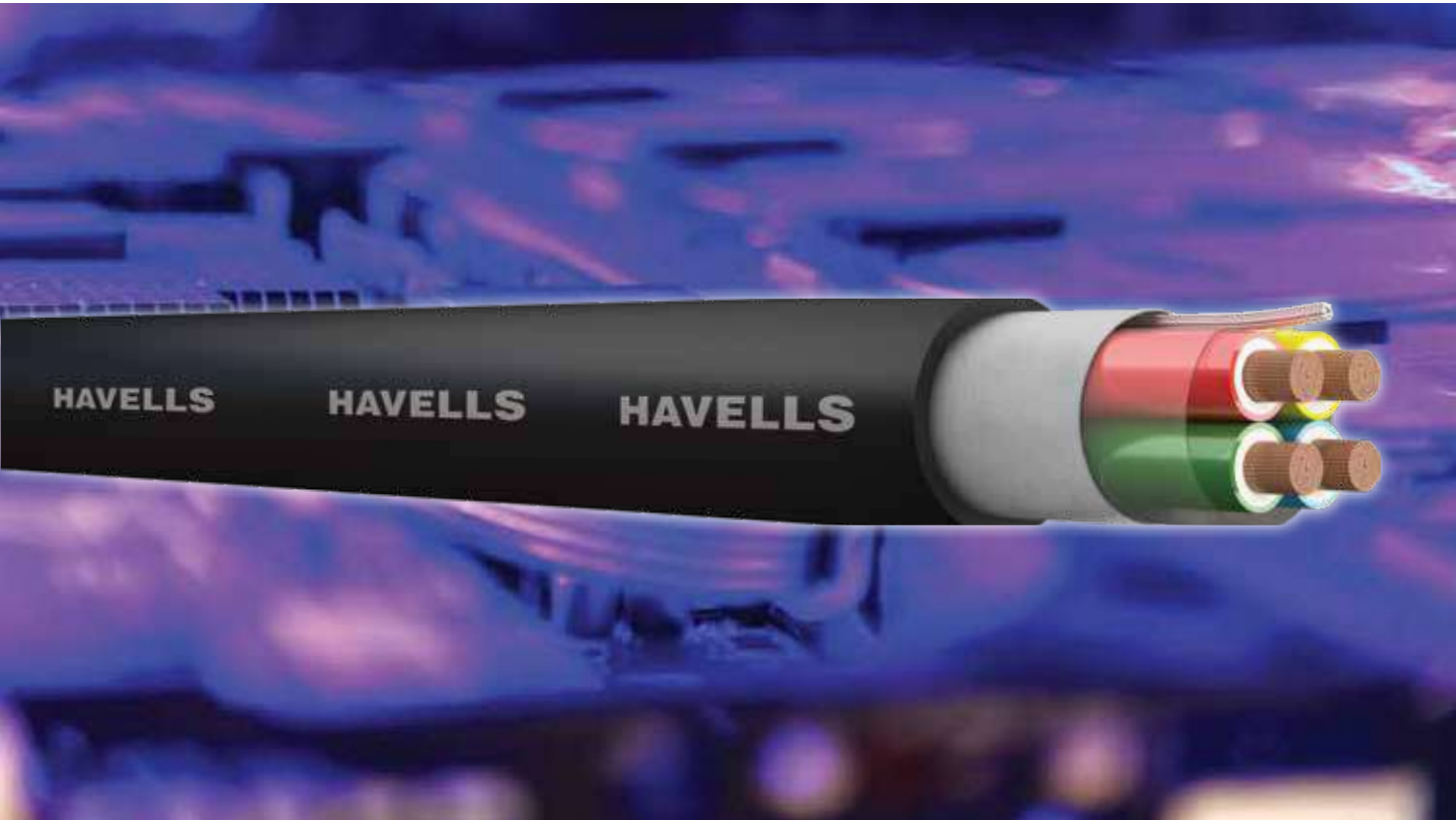
Havells 1100 Volt Flexible ABC Conductor, PVC Type D Insulated, Cores laid up, Overall Shielded by Al-mylar along with ATC drain wire & Overall PVC Type ST-3 Sheathed Cable HSN CODE: 8544
